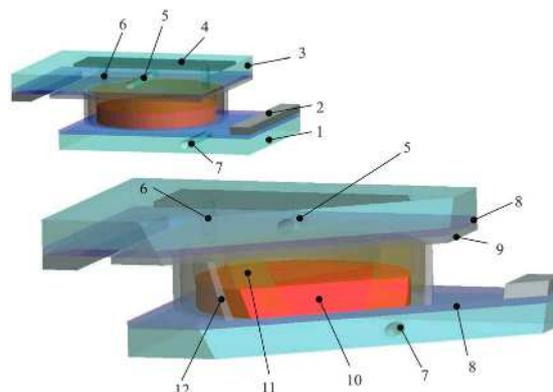
**Fig. 2** Schematic of the manufactured DSC device (not in scale): 1 – photoelectrode glass; 2 – electrical contact; 3 – counter-electrode glass; 4 – filling hole cover; 5 – drilled hole for temperature measurement,  $T_2$ ; 6 – filling hole; 7 – drilled hole for temperature measurement,  $T_1$ ; 8 – TCO; 9 – platinum catalyst; 10 – TiO<sub>2</sub> with adsorbed sensitizer; 11 – electrolyte; 12 – glass frit sealing.
