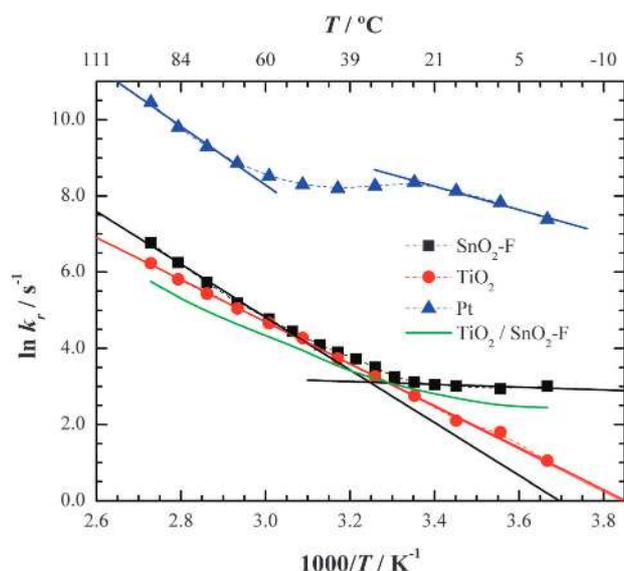
Fig. 14 Arrhenius plot of the recombination reaction (reduction of triiodide) for three types of half-cells: SnO<sub>2</sub>-F, TiO<sub>2</sub> blocking layer and Pt. The green curve represents the average between the TiO<sub>2</sub> and SnO<sub>2</sub>-F curves.
