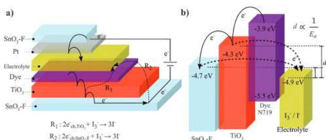
**Fig. 1** (a) Schematic of the working principles at a dye sensitized solar cell; and (b) diagram of energy levels of each functional layer in the DSC. The full arrows represent electron pathways through the device; the dashed arrows represent the main loss reaction mechanisms due to recombination through TiO<sub>2</sub> or SnO<sub>2</sub>-F interfaces ( $R_1$  and  $R_2$ , respectively). The actual energy levels may change upon assembling.
