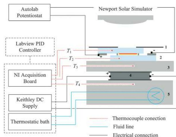
Fig. 3 Experimental setup used for temperature control of an under illumination DSC between  $-5$  °C and 105 °C. 1 – Thermal insulator black mask; 2 – DSC; 3 – aluminum slab; 4 – peltier device; 5 – aluminum slab with drilled thermal fluid circuit.
