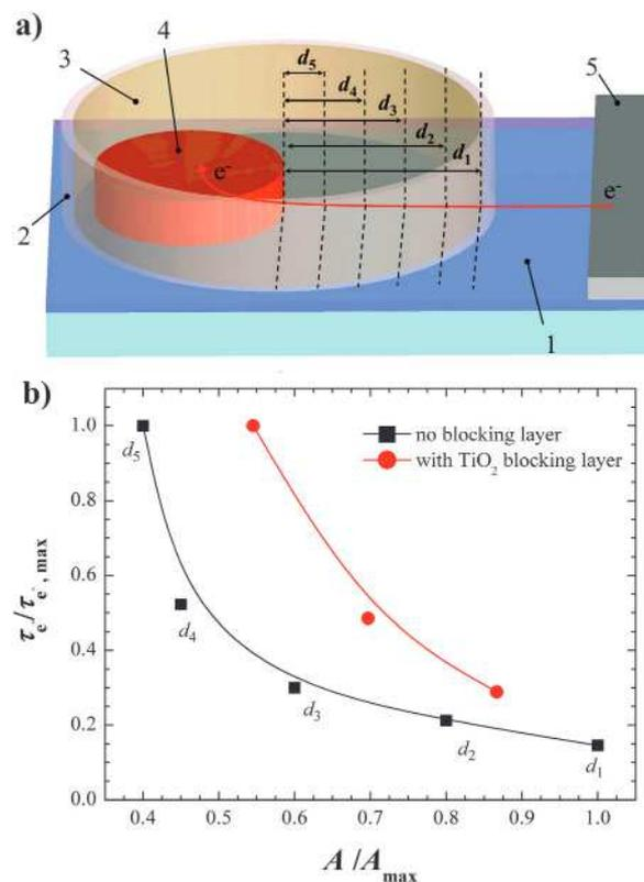
Fig. 11 (a) Schematic showing the methodology to control the FTO/electrolyte exposed reaction interface in the photoelectrode; 1 – TCO; 2 – glass frit sealing; 3 – electrolyte; 4 –  $TiO_2$  with adsorbed sensitizer; 5 – electrical contact; the dashed lines represent the relative positioning of the glass frit sealing. (b) Experimental results of the electron lifetime versus the exposed area of electrolyte to FTO or  $TiO_2$  blocking layer. Lines were added for readability.
