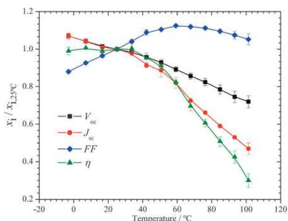
Fig. 6 Performance parameters normalized to the corresponding values 25 °C values ( $V_{OC}$ , 25 °C = 0.77 V;  $J_{SC}$ , 25 °C = 9.5 mA cm<sup>-2</sup>), as a function of the operating temperature. Lines were added for readability.
