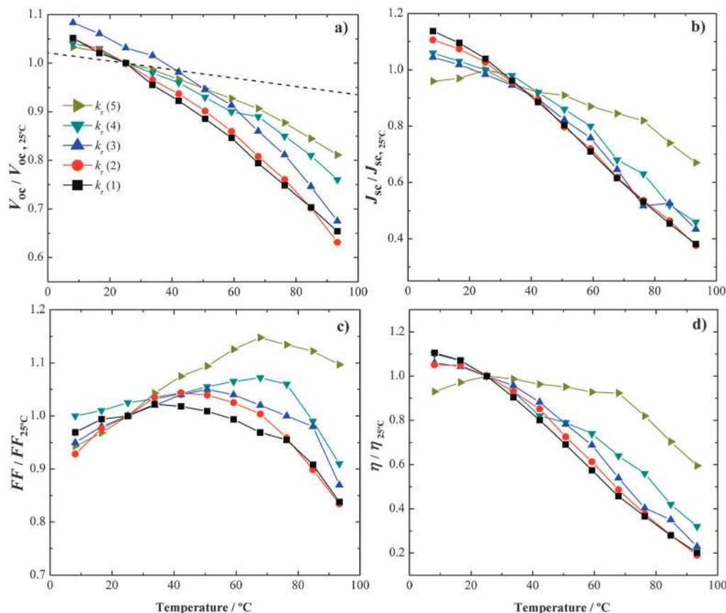
Fig. 12  $I$ - $V$  performance parameters ( $V_{OC}$ ,  $J_{SC}$ , FF and  $\eta$ , a–d respectively) – relative to 25 °C values of five different batches of DSCs differing in the recombination reaction constant  $k_r(i)$ . The black dashed line in (a) corresponds to the theoretical  $V_{OC}$  vs. temperature trend expected for a cell with no recombination (calculated from the Butler–Volmer equation<sup>64</sup>). Lines were added for readability.
