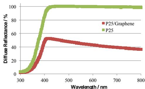
**Figure 2.** Diffuse reflectance spectra of P25 and P25/Graphene composite
