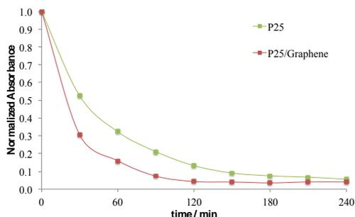
**Figure 1.** Normalized absorbance values for methylene blue degradation during 240 minutes (lines were added to improve the readability).
