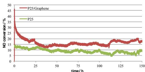
**Figure 3.** NO conversion for P25 and P25/Graphene composite during 150 hours.
