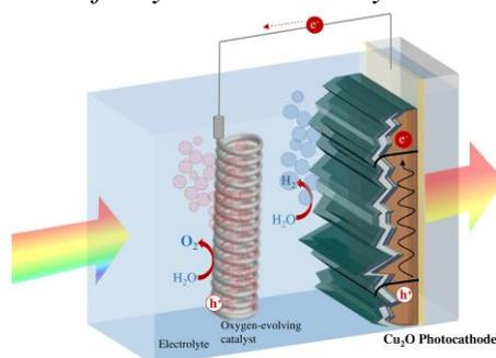
Figure 1. PEC cell based on a Cu<sub>2</sub>O photocathode and a dark counter-electrode.
