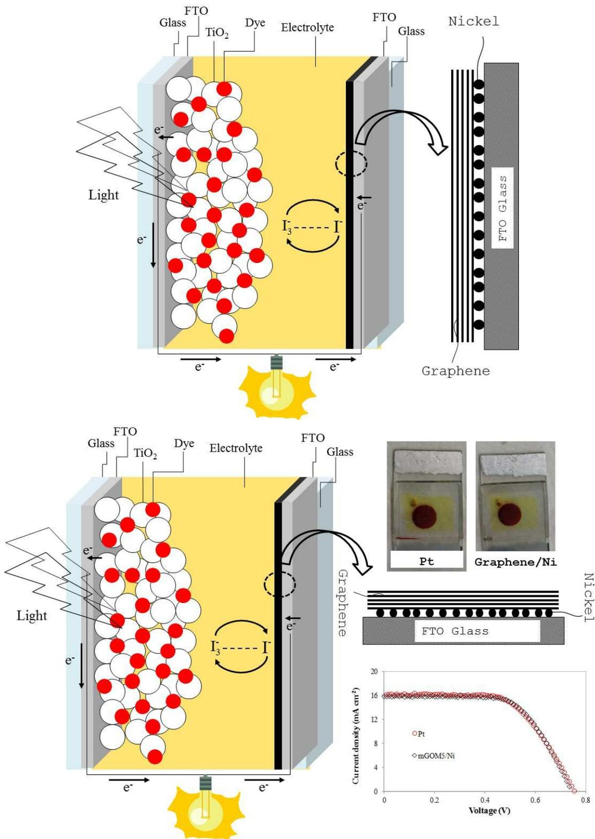
**Figure Legend:** Highly transparent, low cost and easily scalable CEs for DSCs, comprised of a structured graphene film over nickel nanoparticles (graphene/Ni CE), matched the energy conversion efficiencies of the reference platinum CE for liquid-junction iodine and cobalt-based electrolytes.
