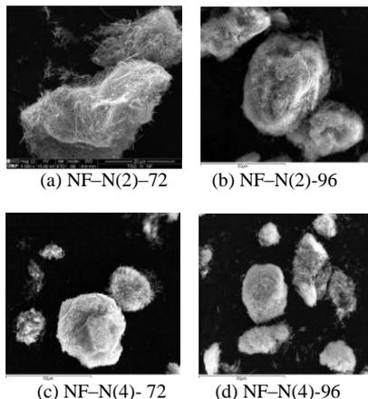
**Figure 2.** SEM images of TiO<sub>2</sub> nanowires synthesized with different % TEA and different synthesis times: a) 2 vol.% of TEA and reaction time of 72 h; b) 2 vol.% of TEA and reaction time of 96 h; c) 4 vol.% of TEA and reaction time of 72 h; d) 4 vol.% of TEA and reaction time of 96 h.
