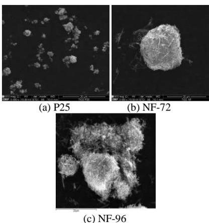
**Figure 1.** SEM images of TiO<sub>2</sub> material synthesized without TEA at different times of synthesis: a) P25; b) reaction time of 72 h; and c) reaction time of 96 h.
