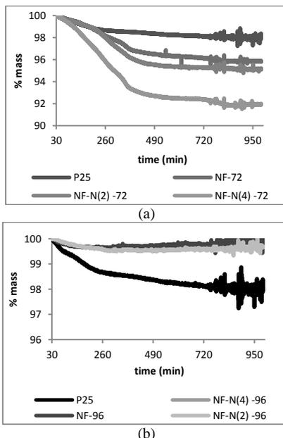
**Figure 3.** TGA comparison of nanowires synthesized with P25 (Evorik) and different TEA percentages with: a) reaction time of 72 h; b) reaction time of 96 h.
