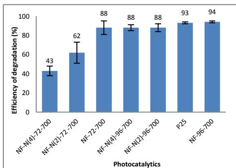
**Figure 5.** Degradation of MB under UV light using the TiO<sub>2</sub> material synthesized, with and without TEA for different synthesis times, measured by the reduction of absorbance in 665 nm after 4 hour, compared with P25.
