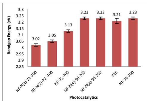
**Figure 4.** Bandgap energy estimated for P25 and nanowires synthesized.
