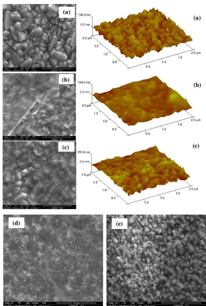
**Fig. 1** AFM and SEM images of (a) the pristine FTO surface, (b) film of oxidized graphene nanoplatelets (mGOM5) deposited on FTO surface prior to thermal annealing and (c) after annealing – notice the moulding effect of the graphene platelets onto the FTO's surface; (d) and (e) SEM images of mGOM5/Ni CE sample after thermal annealing. Concerning Fig. 1e it should
