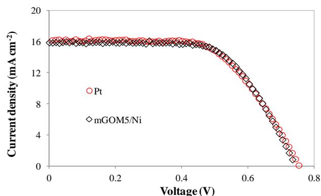
**Fig. 2** I-V characteristics of DSCs assembled with mGOM5/Ni (in water) and with Pt CEs. Measurements carried out at 1 sun ( $100 \text{ mW}\cdot\text{m}^{-2}$ , AM 1.5 G, room temperature). The mGOM5/Ni CEs fabricated using ethanol were not depicted due to overlap with mGOM5/Ni CEs fabricated using water.
