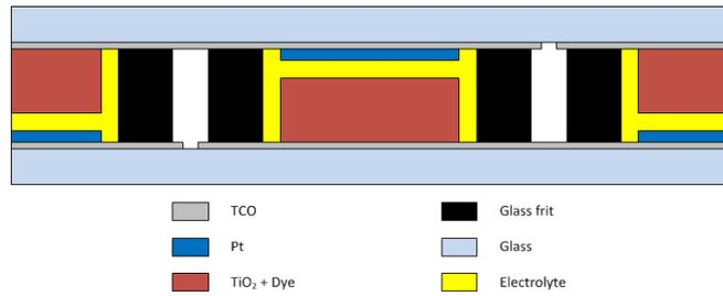
Figure 7 - Double glass-frit cord sealing method (W-configuration).
