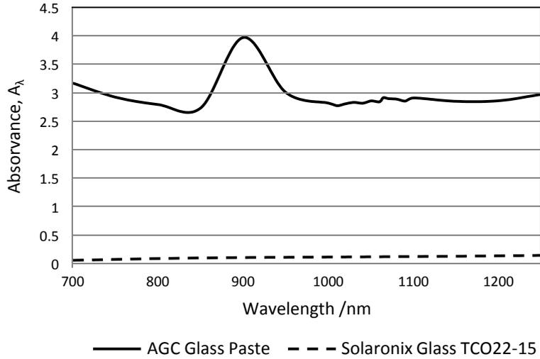
Figure 4 - Absorbance spectrum measured for AGC glass paste and Solaronix coated glass.
