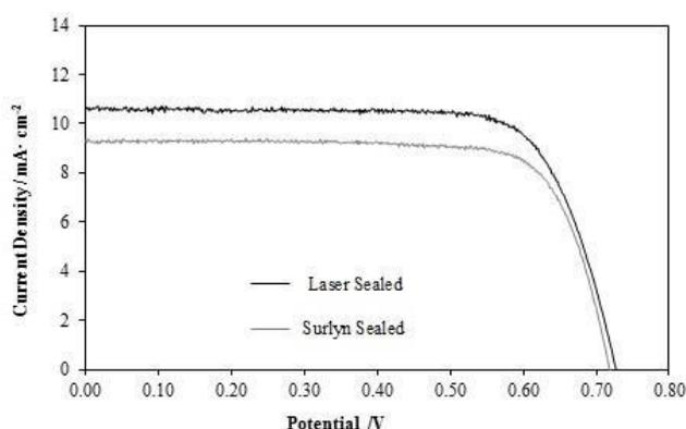
Figure 12 - I-V curves of a glass sealed cell and a cell sealed with thermoplastic polymer Surlyn<sup>®</sup>. (Is – Insiding light intensity; Voc – open circuit potential; Jsc – short-circuit photocurrent; FF – fill factor;  $\eta$  – efficiency)
