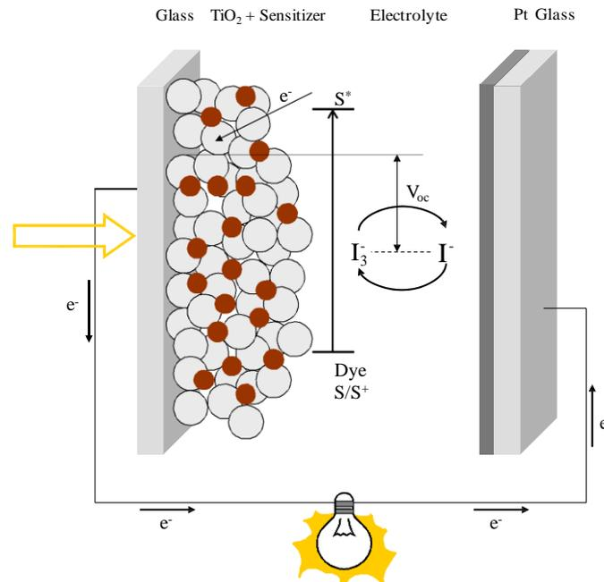
Figure 1 - Scheme of a dye-sensitized solar cell.
