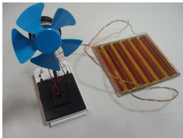
**Figure 10 - Functional DSC module supplying energy for a DC motor.**
