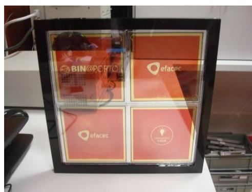
**Figure 11 - Laser assisted glass-frit sealed 300 x 300 mm<sup>2</sup> DSC module.**
