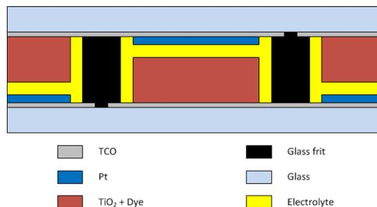
Figure 6 - Shared glass-frit cord sealing method (W-configuration).
