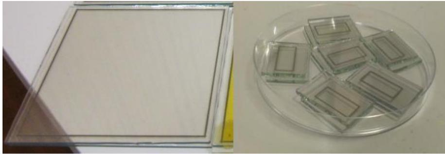
Figure 13 - Empty devices tested according to the standard 61215.
